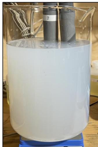
For this commercial 16% PAA product about 24 ppm of product was required per ppm of sulfide.
